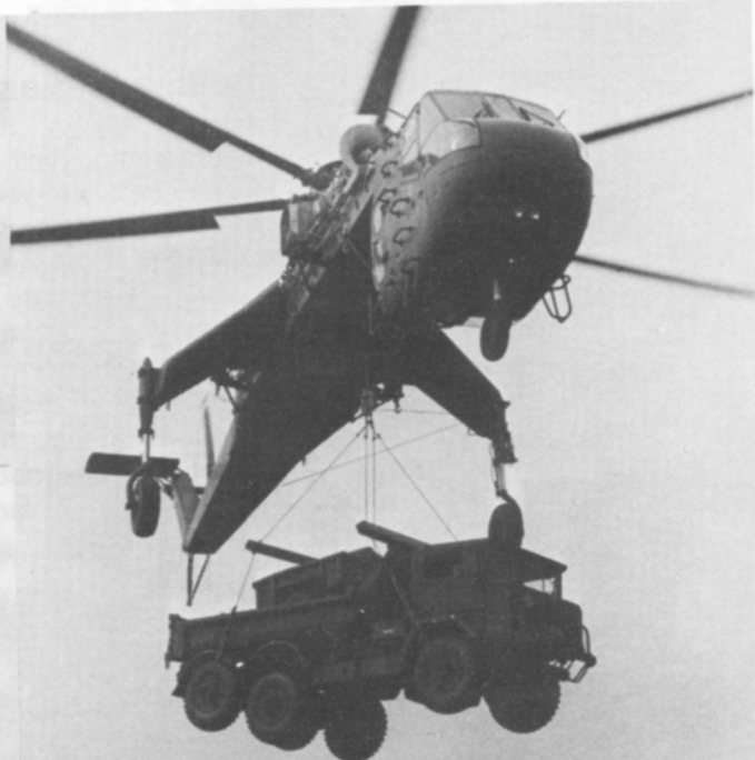
Army Skycrane. Designed and built by our Sikorsky Aircraft Division.
